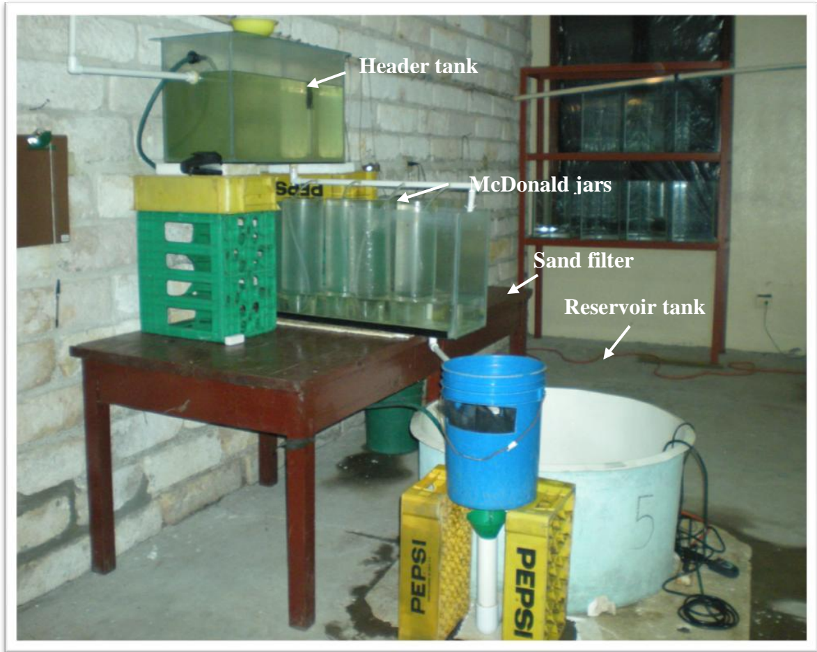
Figure 1. Design of the McDonald jar system used in the artificial incubation of red tilapia eggs in Zamorano, Honduras.
