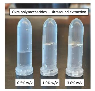
Least Gelation Concentration of okra gum extracted using ultrasound-assisted method.
