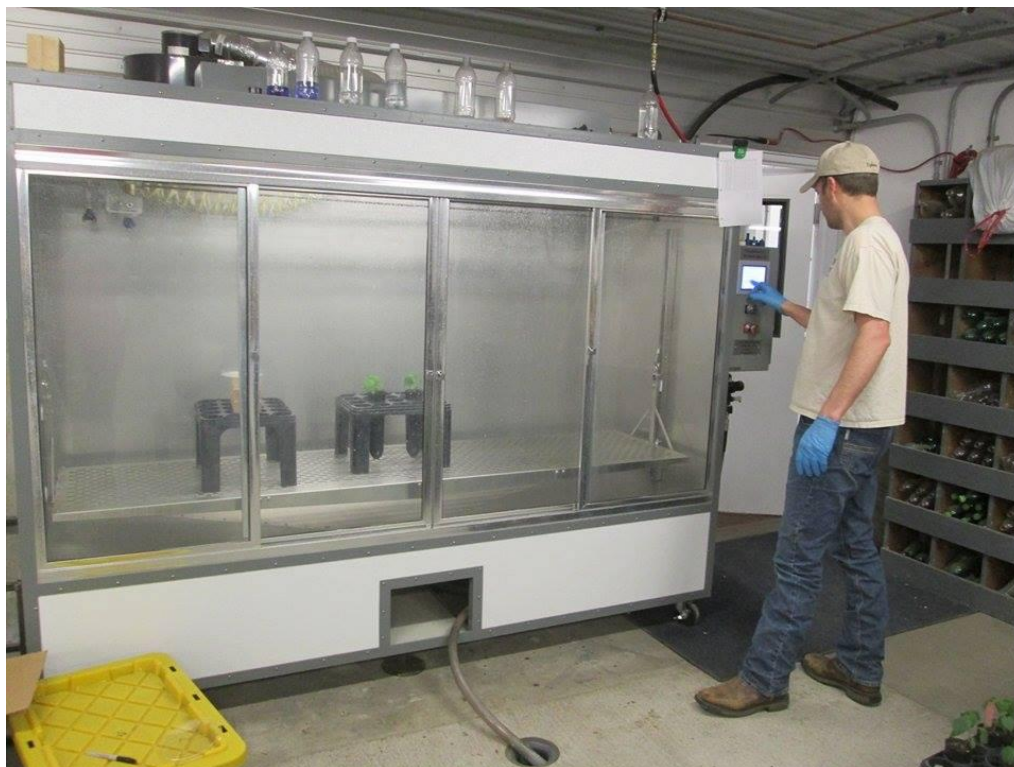
Figura 4. Pista de rociado (Generation III Research Track Sprayer DeVries Manufacturing, Hollandale, MN 56045).
